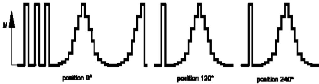
Fig. D.1: Example of preloadings and sequences for torque measuring devices with a minimum 8 steps and U < 0,1\%
