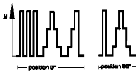
Fig. D.4: Example of preloadings and sequences for torque measuring devices with square drive, a minimum 3 steps and U \geq 1\%
