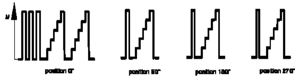
Fig. D.3: Example of preloadings and sequences for torque measuring devices with square drive, a minimum 5 steps, only increasing series and 0,1\% \leq U < 1\%
